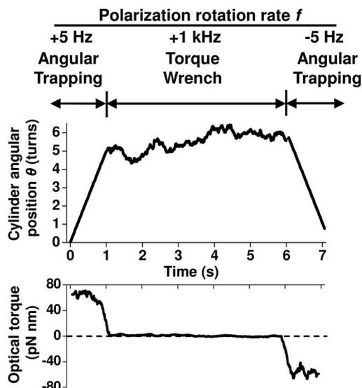
Fig. 3. Demonstration of rapid switching between an angular trapping mode and a torque wrench mode.  $f_{\text{critical}} = 9$  Hz. Polarization rate was set to +5 Hz at  $t = 0$  (angular trapping mode), 1 kHz at  $t = 1$  s (torque wrench mode), and -5 Hz at  $t = 6$  s (angular trapping mode).
